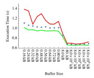
Figure 4: Queue sizes for a matrix multiply application, shown for an individual queue (all queues sized equally). The dots indicate the mean of each observation (each observation is a summary of 1k executions). The red and green lines indicate the  $95^{th}$  and  $5^{th}$  percentiles respectively. The execution time increases slowly with buffer sizes  $\geq 8$  MB, as well as becoming far more varied.
