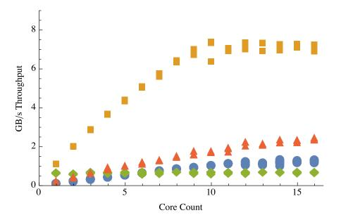
Figure 10: This figure shows the performance of each string matching application in GB/s by utilized cores. This is calculated using a 30 GB corpus searched on the hardware from Table 1. The green diamonds represent the GNU Parallel parallelized GNU grep. The red triangles represent Apache Spark. The blue circles and gold squares represent the Aho-Corasick and Boyer-Moore-Horspool text search algorithms, respectively, parallelized using RaftLib.
