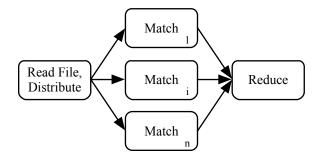
Figure 8: String matching stream topology for both Boyer-Moore-Horpool and Aho-Corasick algorithms. The first compute kernel (at left) reads the file and distributes the data. The second kernel labeled Match uses one or the other algorithms to find string matches within the streaming corpus. The matches are then streamed to the last kernel (at right) which combines them into a single data structure.
